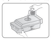
4. Tighten the cap of the water tank in the direction of the CLOSE mark as shown in the picture.
