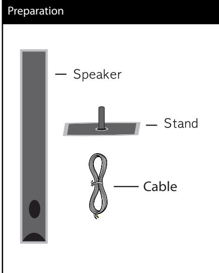
Attach the speaker to the stand, then secure the connection with a supplied screw. Draw the speaker wire through the inside of the stand and also through the hole on the bottom of the speaker.
