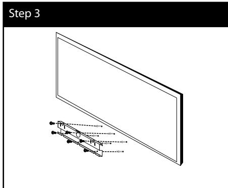
5. Attach the unit bracket to the unit with screws (supplied) as shown in the illustration below.
