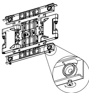
LSW200B/LSW200BG/LSW200BX/LSW200BXG :  $\pm 5\text{mm}(\text{horizontale})$
