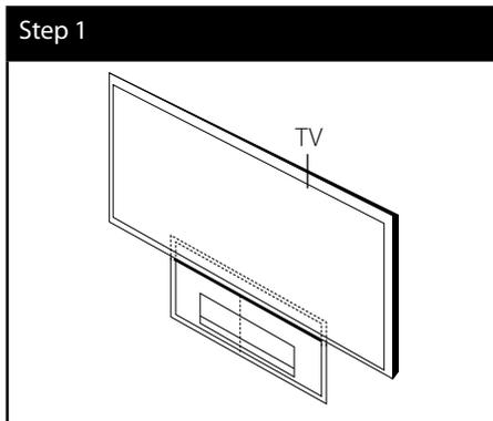
2. When you mount it on a wall (concrete), use the wall plugs (Not supplied). You should drill some holes. A guide sheet (WALL BRACKET INSTALL GUIDE) is supplied to drill. Use the sheet to check the point to drill.
