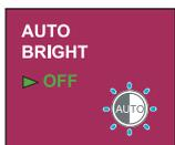
**AUTO BRIGHT** If select on,it automatically controls the brightness of display to best suit the surrounding working environment,providing the optimal viewing condition and maximized user convenience.
