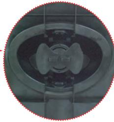
If you can't release the stand base even the locking rib is at a release position, Please push the indicated rib down and retry it.
