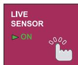
**LIVE SENSOR** This function turns on the button LED for pushing comfortable.When detect the presence of users hand before touch it.
