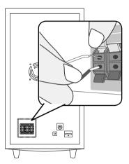
Connect rear speaker wires to the wireless receiver. Use the same method for connecting rear speakers to the wireless receiver unit.
