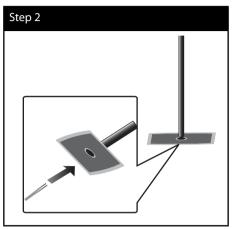
**3.** Draw the speaker wire through the inside of the pole and also through the hole on the bottom of the speaker.
