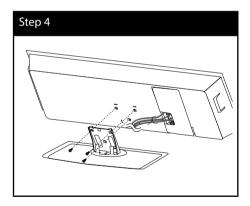
**5.** Arrange the cable with cable holder as shown below.
