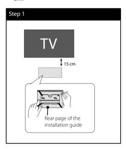
2. When you mount on a wall(concrete), use the wall plugs and screws (Not supplied). Attach the wall bracket on the wall as shown in the illustration below.
