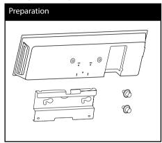
1. You should drill some holes. A guide sheet (rear page of the install guide) is supplied to drill. Use the sheet to check the point to drill.
