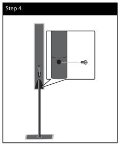
**5.** Connect the speaker wire to the terminal on the speaker.
