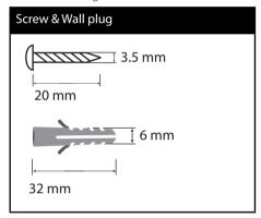
**1.** Attach the wall bracket to the wall with screws as shown in the illustration below.
