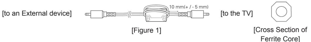
2 Use the ferrite core to reduce the electromagnetic interference in the power cable.
