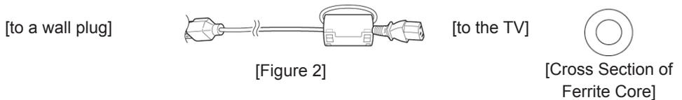
3 Use the ferrite core to reduce the electromagnetic interference in the power cable.
