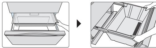
4. Install the whole set of drawer, keeping the rollers of the drawer underneath the rollers of the compartment;
