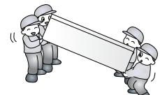
**Carry the refrigerator with the handle bar at the bottom of the front and the top of the rear.**
