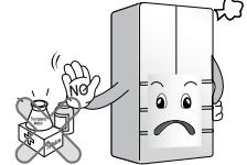
**Do not use the combustible spray near the refrigerator.**
