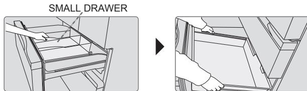
3. Install the white plastic drawer in reverse order, then install the small drawer. Pay attention to the direction when installing the small drawer.
