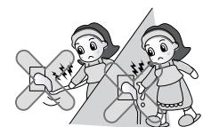
**Remove water or dust from the power plug and insert it with the ends of the pins securely connected.**
