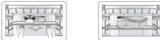
Lift the inside of the shelf and pull it out to remove the shelf. Install the removed shelf at desired position.
