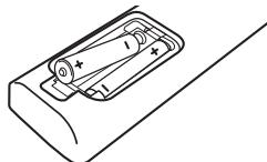
Remove the battery cover on the rear of the Remote Control, and insert two R03 (size AAA) batteries with  $+$  and  $-$  matched correctly.
