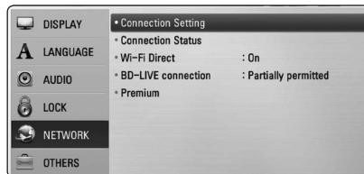
2. The [Connection Setting] menu appear on the screen. Use  $\wedge/\vee$  to select the [Wired] and press ENTER (◎).
