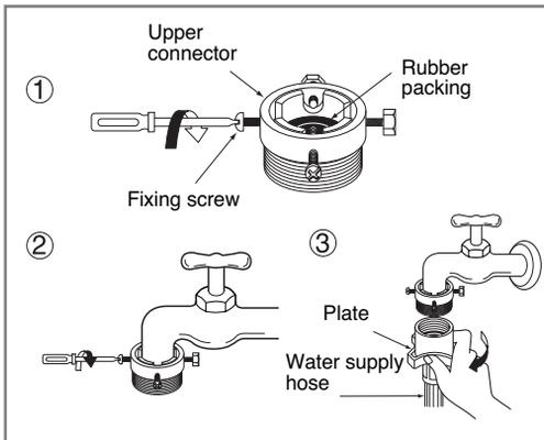
1. Unscrew the adapter ring plate and the 4 adapter retaining screws.
