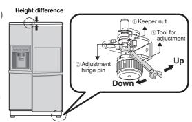
3. After aligning the height of the door, turn the keeper nut in counterclockwise direction tightly.
