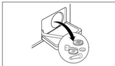
**3.** Remove out any foreign material from the pump filter (3).
