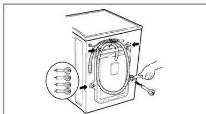
1. To prevent internal damage during transport, the special 4 bolts are locked. Before operating the washer, remove the bolts along with the rubber bungs.
