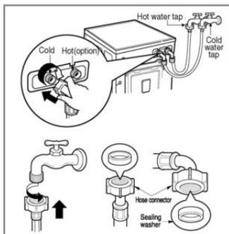
► Water supply pressure must be between 30kPa and 1000kPa (0.3~10kgf/cm<sup>2</sup>)
