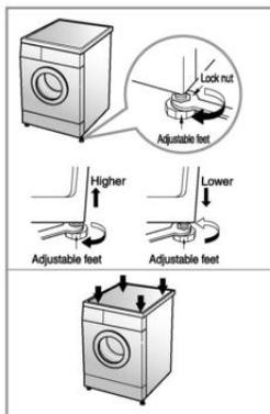
2. If the floor is uneven, adjust the adjustable feet as required. (do not insert pieces of wood etc. under the feet)
