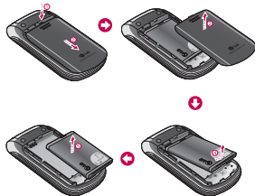
To insert the SIM card
