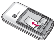
To remove the USIM card
