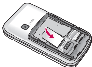
To insert the USIM card
