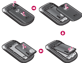
To insert the SIM card
