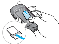
To remove the SIM card
