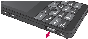
Remove the memory card
