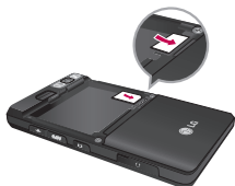
To insert the SIM card
