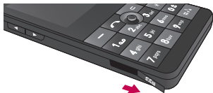
Open the memory card slot
