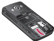
To insert the USIM card To remove the USIM card
