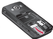
To remove the USIM card
