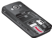
To insert the USIM card
