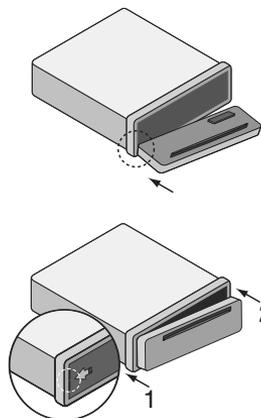
1 Align the left side of the panel with the stopper.
