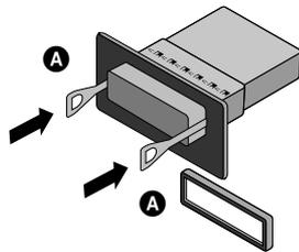
If there is already an installation sleeve for the receiver unit in the dashboard, it must be removed.
