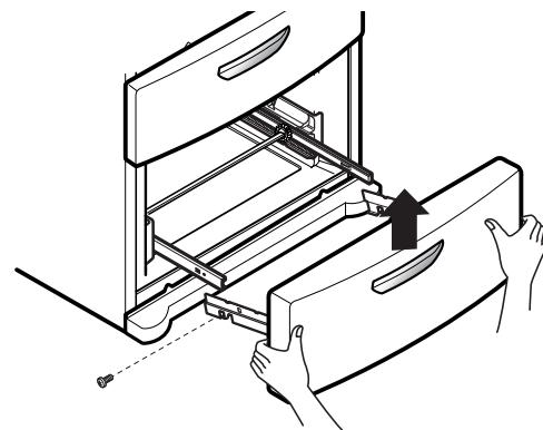
4 With both hands, flex the center bar enough to allow the gears on both ends to release from the track.
