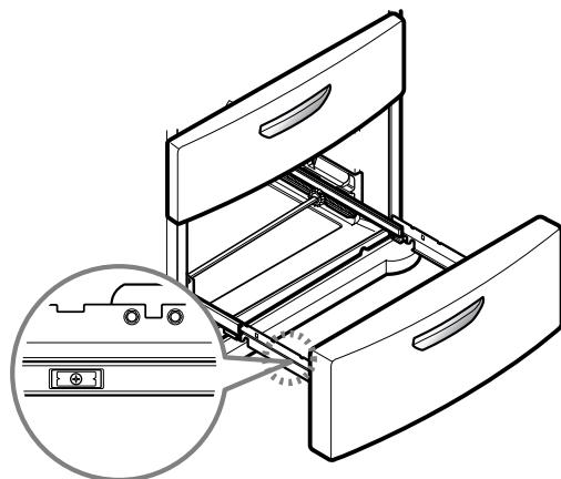
3 Grasp the drawer on each side and pull it up to separate it from the rails.
