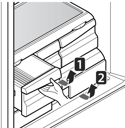
To install, slightly tilt up the front, insert the drawer into the frame and push it back into place.
