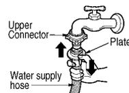
• In case the diameter of the tap is large remove the guide plate.
