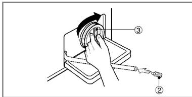
4. After cleaning, turn the pump filter (③) clockwise and insert the drain plug (②) to the original place. Close the lower cover cap.
