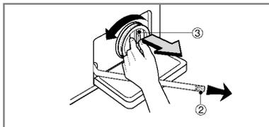
2. Unplug the drain plug (②), allowing the water to flow out. At this time use a vessel to prevent water flowing on to the floor. When water does not flow any more, turn the pump filter (③) open to the left.
