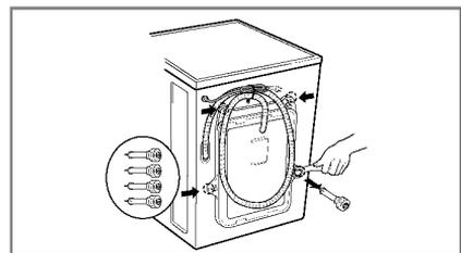
3. Take out the 4 bolts along with the rubber bungs by slightly twisting the bung. Keep the 4 bolts and the spanner for future use.
