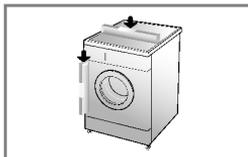
1. Adjusting the washing machine level properly prevents excessive noise and vibration.
