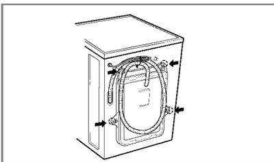
1. To prevent internal damage during transport, the special 4 bolts are locked. Before operating the washer, remove the bolts along with the rubber bungs.
