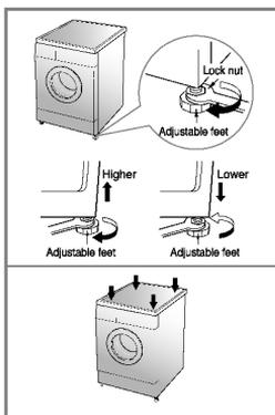
2. If the floor is uneven, adjust the adjustable feet as required. (do not insert pieces of wood etc. under the feet)
