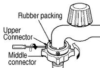
3. Connect the water supply hose to the middle connector, pushing the plate down.
