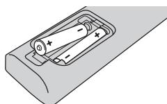
Remove the battery cover on the rear of the Remote Control, and insert two R03 (size AAA) batteries with  $+$  and  $-$  matched correctly.
