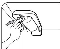
**NOTE: Replacing the water filter causes a small amount of water (around 25ml) to drain. Place a cup under the front end of the water filter cover to collect any leaking water. Hold the water filter upright, once it is removed, to prevent any remaining water from spilling out of the water filter.**
