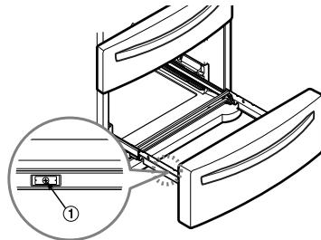
3 Holding both sides of the door pull up to separate the door from the rails.
