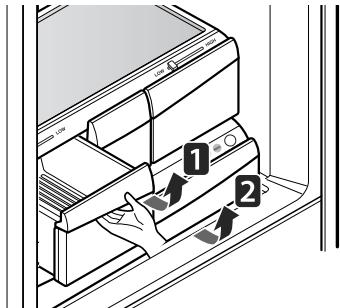
To install, slightly tilt up the front, insert the drawer into the frame and push it back into place.
