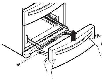
4 With both hands, hold each rail and push it in to allow both rails to slide in simultaneously.
