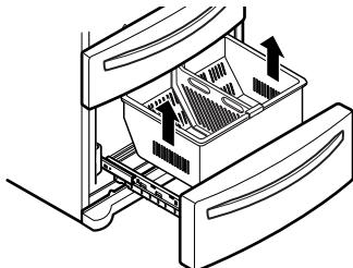
2 Remove one white screw ① on each side of the rails.
