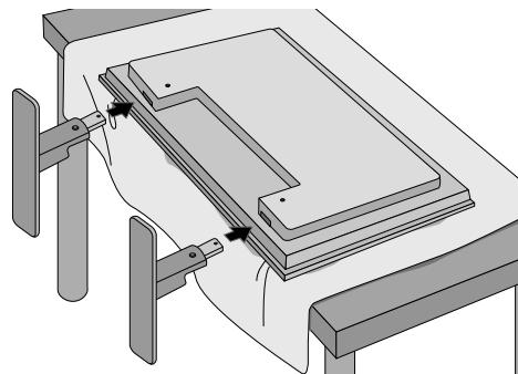
3. Use the screws to secure the stand on the rear side of the product as shown in the diagram.
