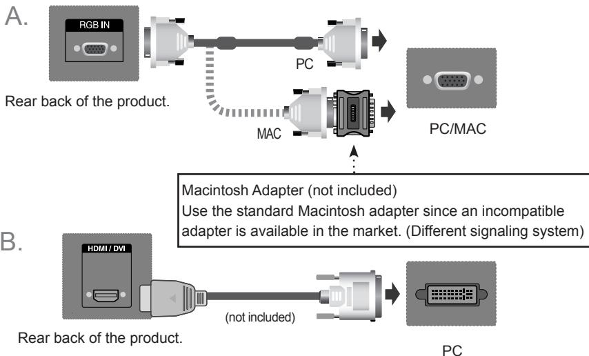
\* User must use shielded signal interface cables (D-sub 15 pin cable, HDMI-DVI cable) with ferrite cores to maintain standard compliance for the product.
