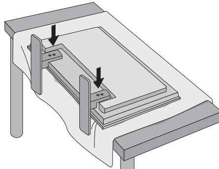
3. Use the screws to secure the stand on the rear side of the product as shown in the diagram.
