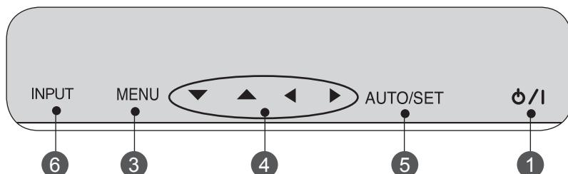
1 **On/Off button** Press this button to turn on the power. Press this button again to turn it off.
