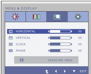
**PHASE** To adjust the focus of the display. This item allows you to remove any horizontal noise and clear or sharpen the image of characters.
