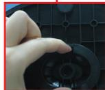
When you desire to disintegrate the monitor from the stand base, use a coin to turn the screw counterclockwise.
