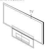
When you mount it on a wall (concrete), use the wall plugs (Not supplied). You should drill some holes. A guide sheet (WALL BRACKET INSTALL GUIDE) is supplied to drill. Use the sheet to check the point to drill.
