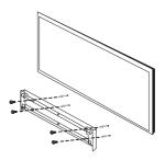
5. Hang the main unit onto the brackets, as shown below.
