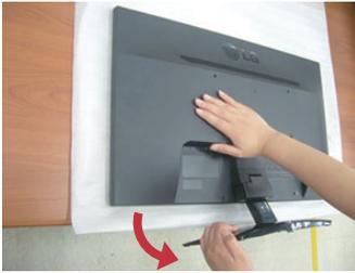
4. Use a coin on the back of the Stand Base and turn the screw anticlockwise to loosen.
