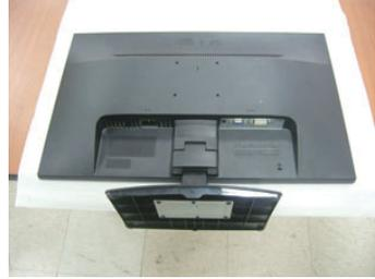
3. Remove the Stand Body and Stand Base from product in correct direction as shown in the picture.
