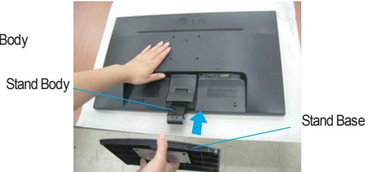
4. Use a coin on the back of the stand base and turn the screw clockwise to tighten.
