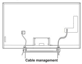
2 Install the cable holder as shown.
