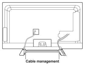
2 Gather and bind the cables with the cable holder on the TV back cover.
