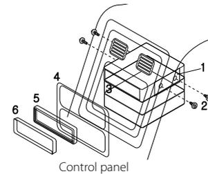
1. Slide the unit into the ISO-DIN frame.
