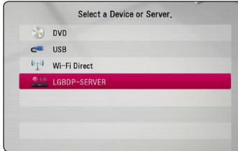
To select a server from the device list, files or folders must be shared by DLNA server from the connected Wi-Fi Direct™ device.
