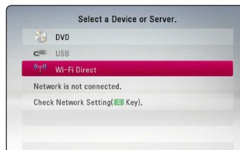
5. Select a Wi-Fi Direct™ device on the list using **A/V**, and press ENTER (O).
