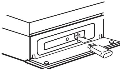
When you connect the USB device on the HOME menu, the player plays a music file contained in the USB storage device automatically. If the USB storage device is containing various types of files, a menu for the file type selection will appear.
