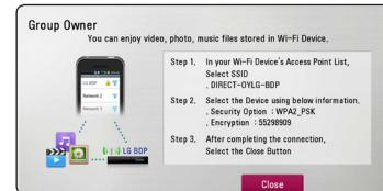
6. On your Wi-Fi device, make a network connection to this player, using [Network name (SSID)], [Security Option] and [Encryption] at step 5 above.
