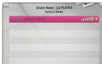
If the Wi-Fi Direct™ device supports the PIN Code configuration method based on WPS(Wi-Fi Protected Setup), select a device on the list and press yellow (Y) coloured button. Note the PIN number on the screen. And then, enter the PIN number on a setting menu of the device to connect.
