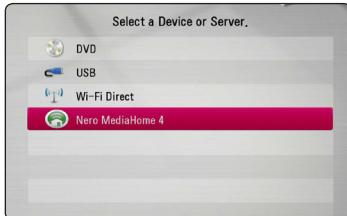
To select a server from the device list, files or folders must be shared by DLNA server from the connected device.
