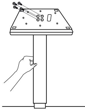
3. Attach the speaker to the pole, then secure the connection with a supplied screw.
