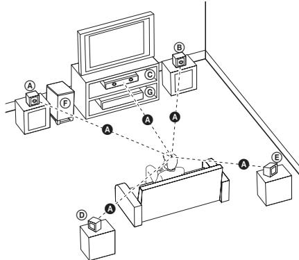
Ⓐ Front left speaker (L)/ Ⓑ Front right speaker (R): Place the front speakers to the sides of the monitor or screen and as flush with the screen surface as possible.
