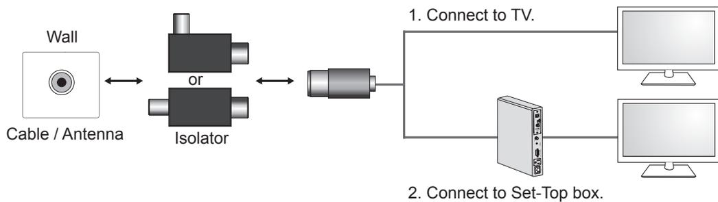
Connect one end of the isolator to cable/antenna jack and the other to TV set or set-top box.
