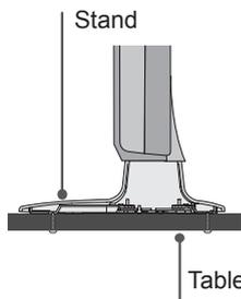
Screws: M4 x L (\*L: Table depth + 8-10 mm)
