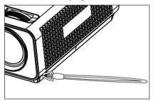
3 Fix the strap at the hole of the projector into the hole of the lens cap, and then pass the lens cap through the strp lasso.
