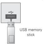
To disconnect a USB storage device, make sure to end the connection properly to prevent damages to the projector or files.
