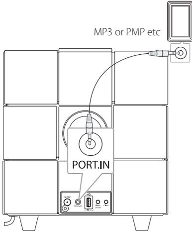
1. Connect the external device to the **PORT.IN** connector of the unit.
