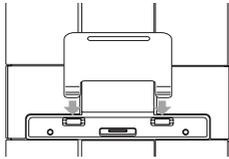
1. Connect the iPod/iPhone/iPad firmly. When this unit is connected to power, your iPod/iPhone/iPad is automatically turned on and starts recharging even in standby mode.
