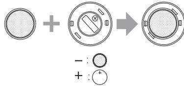
3. Put the battery compartment lid on the remote control and turn it clockwise to close.
