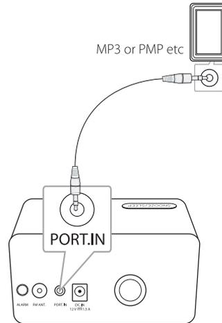
1. Connect the external device to the **PORT.IN** connector of the unit.
