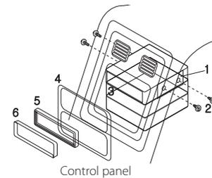
1. Slide the unit into the ISO-DIN frame.
