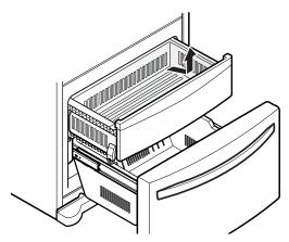
To reinstall, pull out and fully extend both rails. Insert the end of rib in the bracket at left and right. Making sure that the guides at the front are lined up properly, gently push down on both sides.
