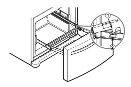
3 Lower door into final position and tighten the screws.
