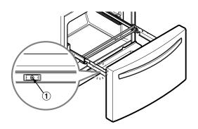
3 Holding both sides of the door pull up to separate the door from the rails.
