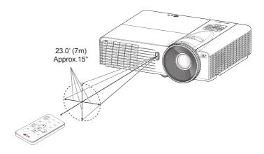
Point the remote control toward the projector (Infrared Remote Receiver) when pressing any button. Maximum operating range for the remote control is about 23.0′ (7m) and 30° in front of the projector.
