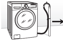
Connecting the drain line
