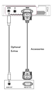
You can connect the audio cable without using a gender as shown in the illustration above.
