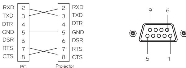
[Figure 1] RS-232 Connection Diagram
