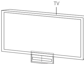
2. When you mount it on a wall (concrete), use the wall plugs (Not supplied). You should drill some holes. A guide sheet (Wall Mount Bracket Installation Template) is supplied to drill. Use the sheet to check the point to drill.
