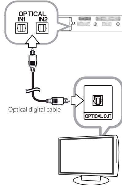
2. Set up LG Sound Sync (Optical) on the TV. Refer to the TV's instruction manual.
