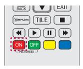
3 If you press the left/right buttons or the red ON button for PICTURE ID repeatedly, the Picture ID toggles between OFF and 0 to 4. Assign the Set ID as you like.
