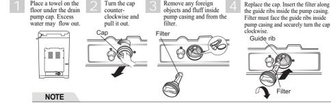
• Check if water leaks after reassembling. (The Rubber ring is in the cap)
