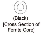
2 Use the ferrite core to reduce the electromagnetic interference in the cable.
