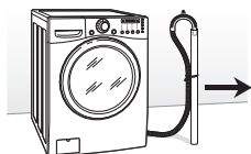
Connecting the drain line
