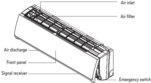
\* Do not remove the film. Please keep the protective film of emergency switch. This is used to protect the product from ESD damage.
