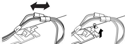
3 Turn ① around to release lock and raise hinge up.
