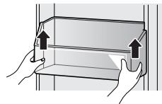
To refit the basket, align both sides of the basket with the guides and push it down until secure.
